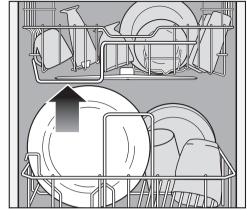
The guide at the front of the upper basket (arrow) shows the maximum height of items that can be placed in the lower basket. Items taller than this will block the middle spray arm.
